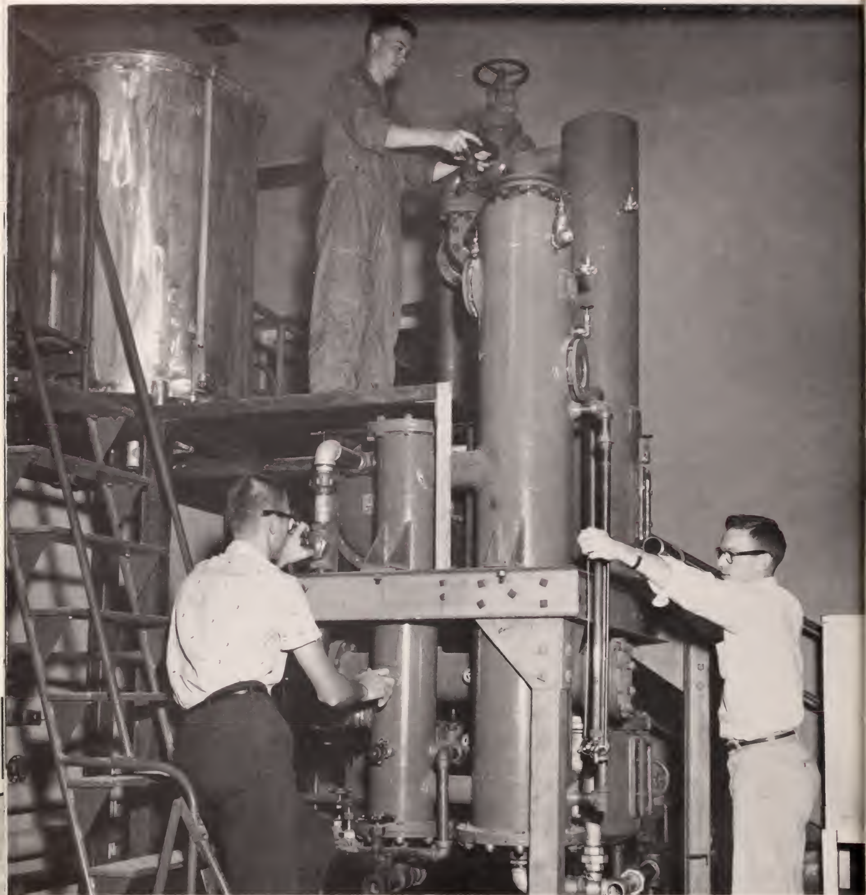
Rudy Kittlitz, Bill Cole, and Oscar Wall work on the double-effect evaporator in the Chemical Engineering Building. This set-up is used to make concentrated solutions from diluted ones. It could be said that they are concentrating on the concentrating apparatus.
